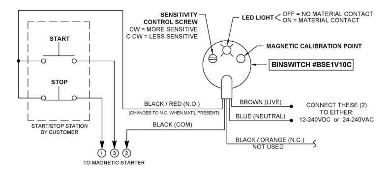
The conveyor should only be able to operate when the LED is OFF!
